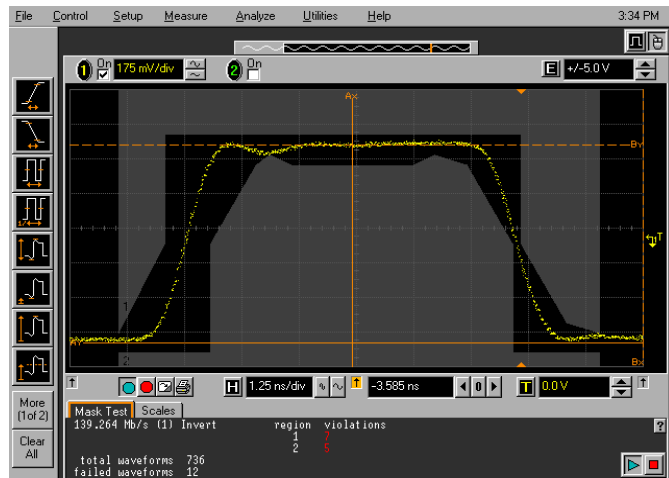
140Mb/s All Ones (inverted) Mask Test
