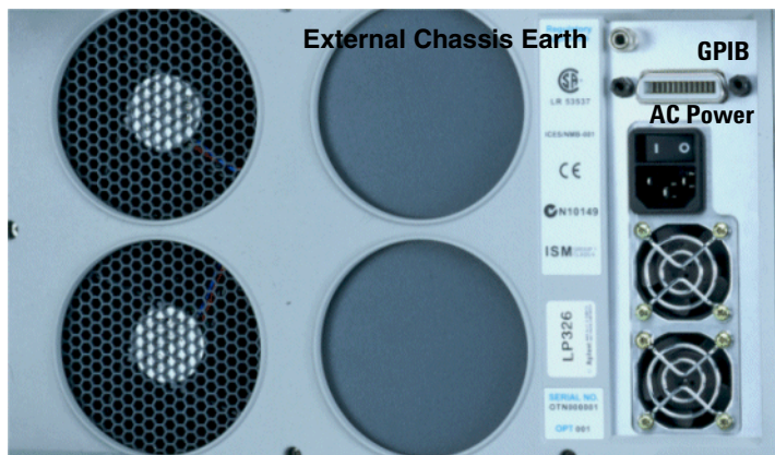
Figure 1 Earthing terminal - rear panel
